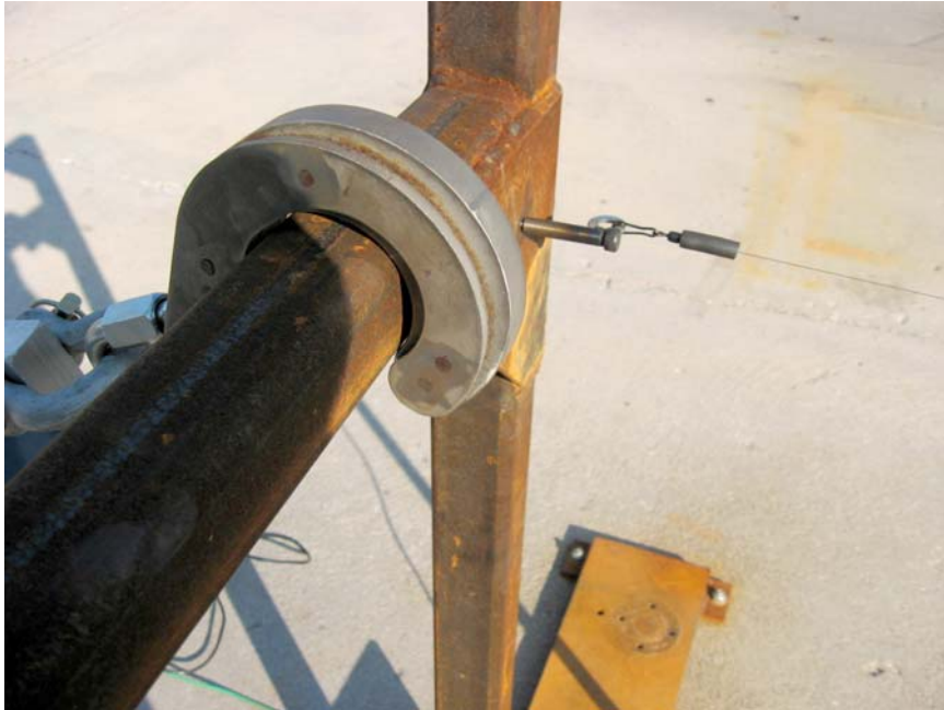
Fig. 3 - A close-up view of the load and deflection measurement point is shown. The deflection was measured from the back in the first test.
