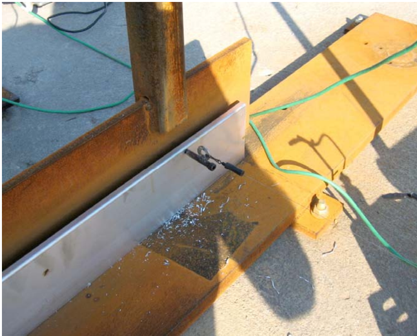
Fig. 4 - A close-up view of the deflection measurement point on the shoe is shown. The deflection was measured from the back in the first test.
