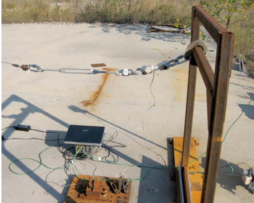
Fig. 1 - An overall view of the first test setup is shown. The load was applied near the corner of the rail.
