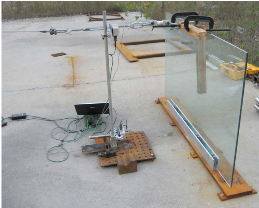
Fig. 11 - An overall view of the fourth test setup is shown. The load was applied near the middle of the glass panel.
