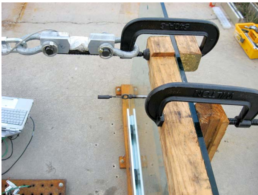
Fig. 12 - A close up view of the load and deflection measurement point is shown. Wood blocks were used to distribute the load. Deflection was measured from the front in the fourth test.
