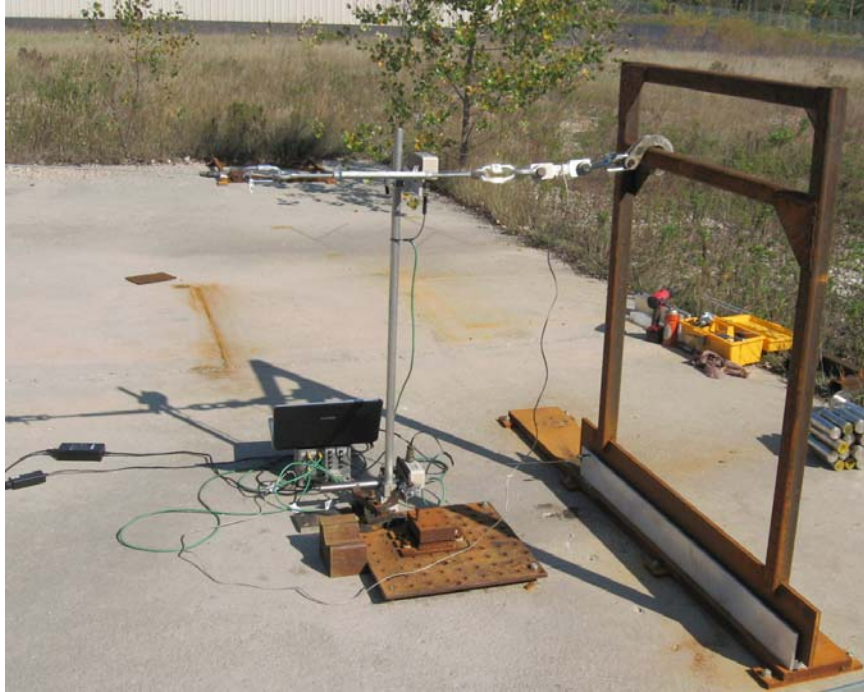
Fig. 5 - An overall view of the first test setup is shown. The load was applied near the corner of the rail.
