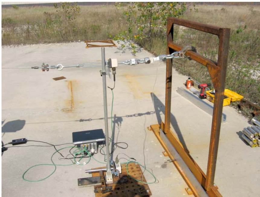
Fig. 8 - An overall view of the third test setup is shown. The load was applied near the middle of the rail.
