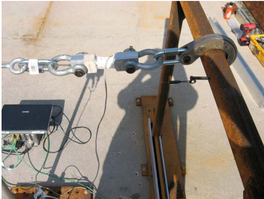
Fig. 9 - A close up view of the load and deflection measurement point is shown. The deflection was measured from the front in the third test.
